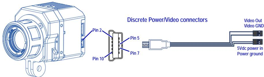
Simply plug the chosen cable into the mini-USB port on the FLIR Vue Pro, connect the power plug to an appropriate regulated power supply, and the video plug to the video transmitter.
