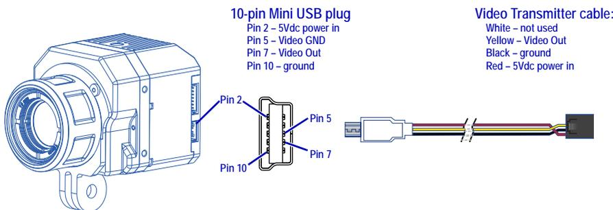
Another example of a compatible cable which provides discrete connectors for power and video is shown below.
