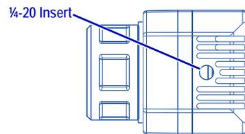
FLIR Vue Pro has two threaded mounting holes on each side, as well as on the camera bottom.
